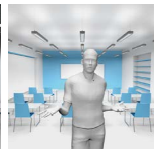
For the correct modelling of the faces it is important to ensure in the classrooms sufficient cylindrical illuminance amounting 150 lux. The suspended luminaires with the direct and indirect characteristic of the luminous flux distribution which eliminate forming undesirable shadows and at the same time do not cause glare are the optimal solution.
