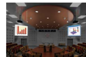
LIGHTING SCENE 3: During presentation with an overhead projector the general lighting is dimmed and lights at 10%.
