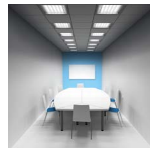
The classical solution of the lighting with recessed luminaires with a parabolic louvre ensures sufficient illumination of the workplace but the upper parts of the walls and the ceiling remain dark. Such illumination causes a feeling of a cave effect and makes the room optically smaller.
