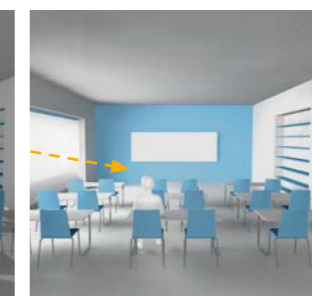
Fitting the windows with an effective system of blinds belongs among the basic measures how to avoid the direct glare from sunshine.
