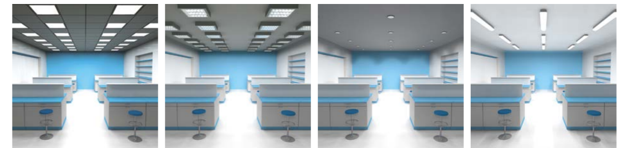
The harmonious distribution of brightness in a space can be influenced by a selection of luminaires. By using luminaires with direct distribution of the luminous flux (Figure 1-3) we don't achieve sufficient illuminance of vertical surfaces, which causes a cave effect. It can be avoided by using luminaires with a very wide luminosity curve. (Fig. 4).
