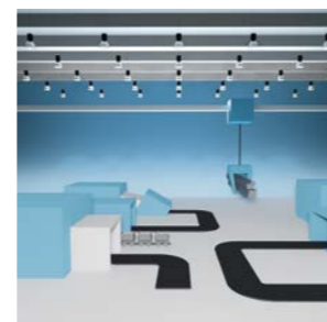
In production halls with standard height of the walls it is suitable to use linear luminaires with the direct characteristic of the luminous flux. To obtain the standard stated levels of the maintained illuminance it production halls with non standard height of the walls (6 m and more) it is important to choose luminaires that can be used in different mounting height
