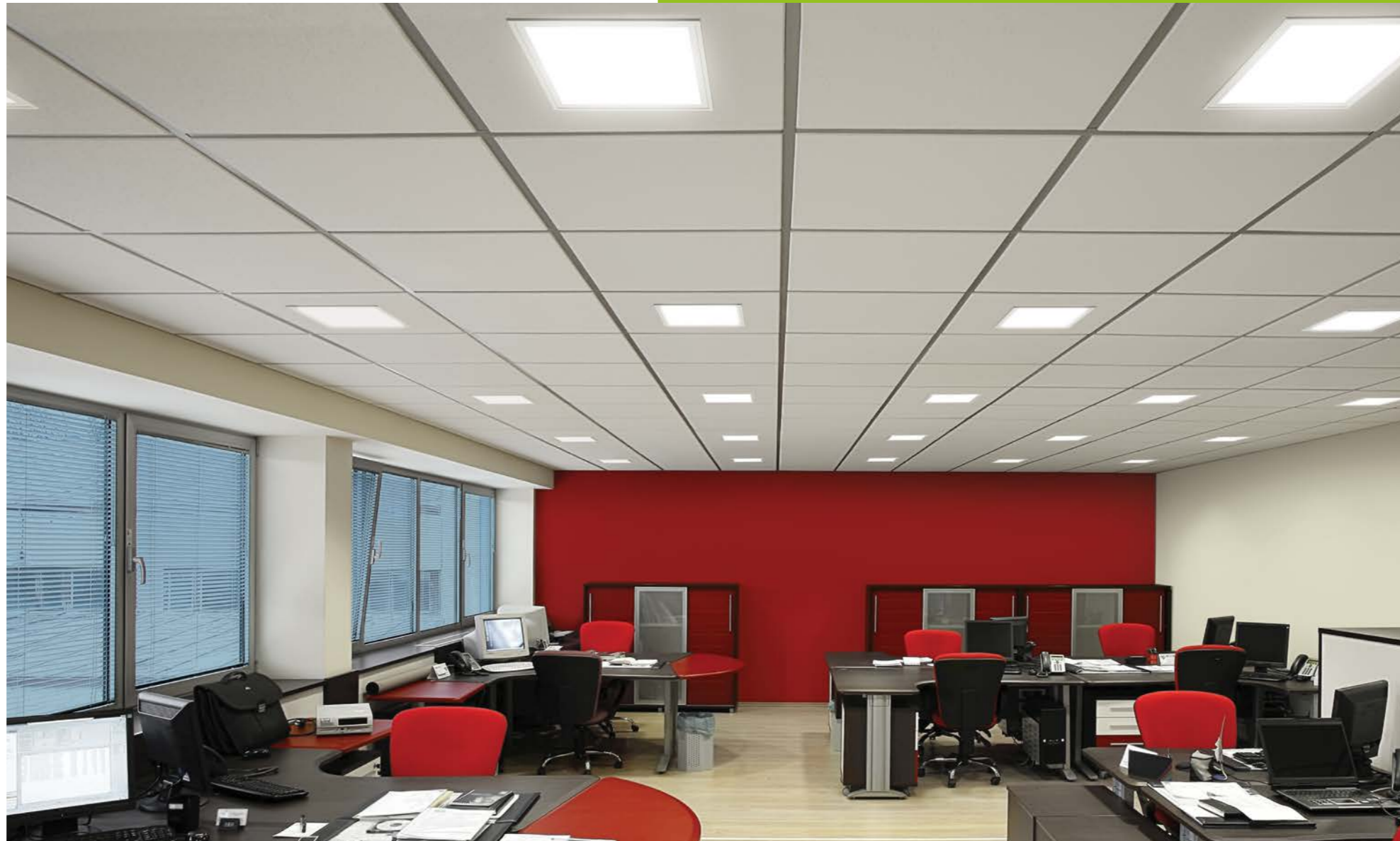
In the architects' offices, rooms determined for technical drawing and in CAD rooms the correct colour rendering is of exceptional importance therefore, usage of light sources with colour rendering index 90 is recommended.
