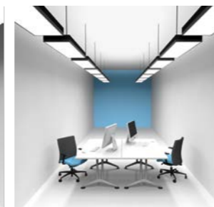
Optimal values for distribution of brightness in the space can be achieved by using suspension luminaires with both direct and indirect characteristics of the luminous flux distribution.
