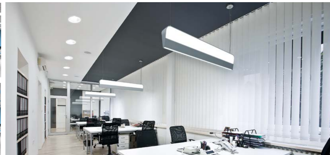
The lighting system has to be adapted to the structure of the space in the open space office. Increased demands are placed on the lighting uniformity that should prevent a strong exposure and rise of sharp shadows.
