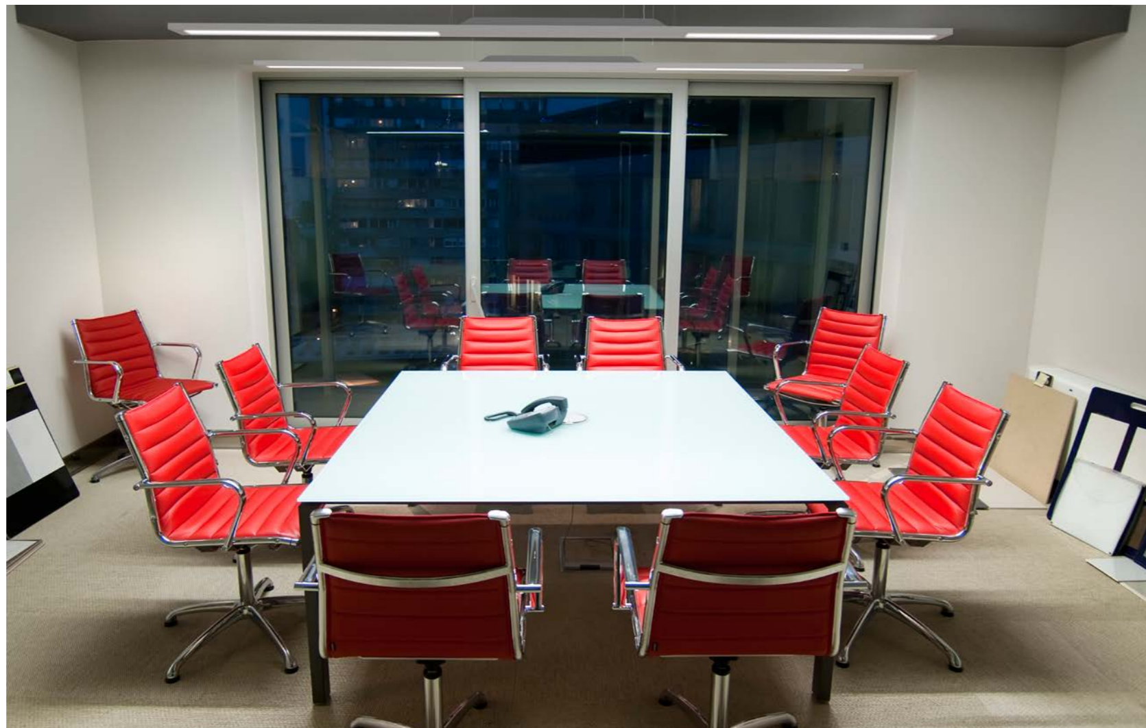
A suspended LED luminaire with direct and indirect distribution of diffuse light through microprism is an ideal solution for the office spaces.
