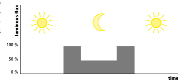
A Single phase switching with twilight sensor.
