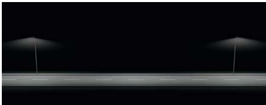
D Luminaires with high performance optics that emit light laterally over a large distance, ensuring that the road is evenly illuminated, and visual acuity maintained.
