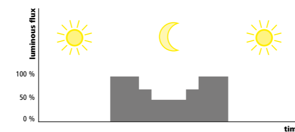
B Single phase switching with twilight sensor.
