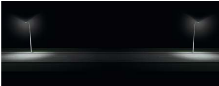
C Conventional luminaires that illuminate unevenly, creating 'hot spots' that reduce visual acuity.
