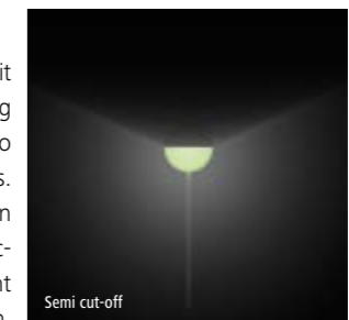
B Still the most common type found and usually pole mounted cobra head luminaires that do not emit light upwards. As the optics drop below the luminaire housing, light is distributed well over larger areas making them ideal for high mounting, but as much as 5% of the light it emitted above 90°.
