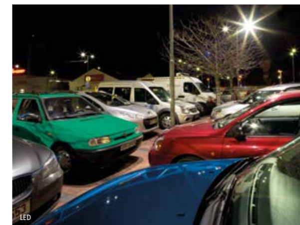
Colour perception of high-pressure sodium compared to LED with CRI ≥ 70.
