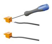
**2.** Using a flat-headed screwdriver, press down the upper jaws of the plug and insert the sensor cable wires into the lower jaws. Fasten the wires by releasing the upper jaws.
