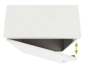
**1.** Fix the door sensor to the streetlight cabinet wall and its doors, so the closed state in an closed state the distance between the sensors does not exceed 10 mm.
