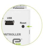
If there is a need to change configuration of the device, it is necessary to restart the device to factory settings using button Reset (press and hold for 10 sec).
