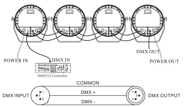
Termination reduces signal errors and to avoid signal transmission problems and interference. It is always advisable to connect a DMX terminal. (Resistance 120 ohm 1/4W)between pin2(DMX-)and
